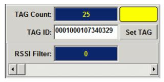
RSSI filter: Adjust RSSI filter (0~255) to reject TAG which have low RSSI signal in this utility program.
