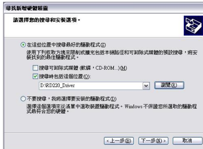
Figure 5 Browse to folder "RD220_Driver" in CD or where the driver is located
